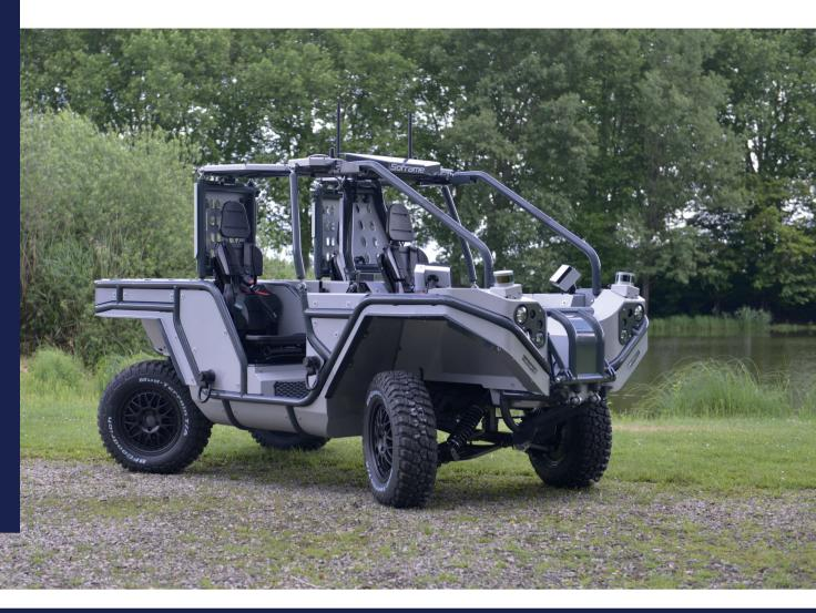
4x4 light, all-terrain vehicle, high speed, modular with open cab.
