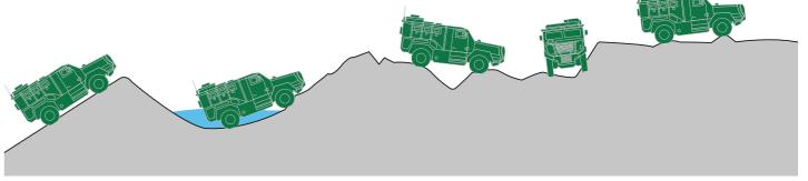
Slope Fording Trench Side Slope Step 60 % 800 mm 900 mm 30 % 400 mm
