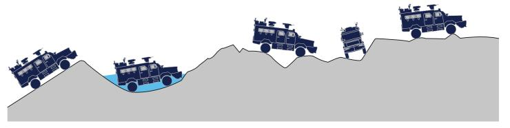
Slope Fording Trench Side Slope Step 40 % with front blade 600 mm 900 mm 30 % 400 mm **60** % without front blade
