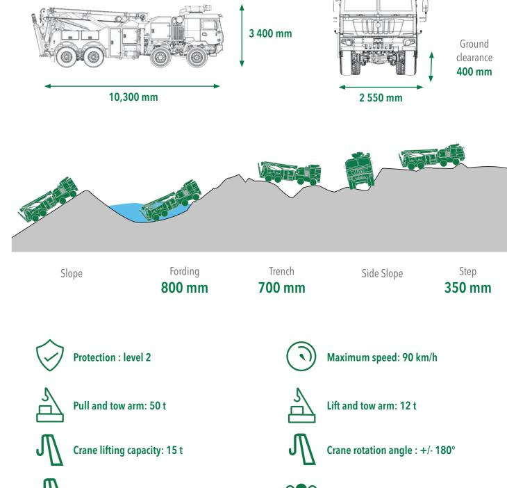
**The PPLD heavy multi-purpose recovery truck** is the French army's benchmark all-terrain recovery vehicle. It is intensively **used for missions abroad** in particular. Its recovery system has a main **18-tonne haulage winch** and an auxiliary winch enabling it to **cope with all situations**.
