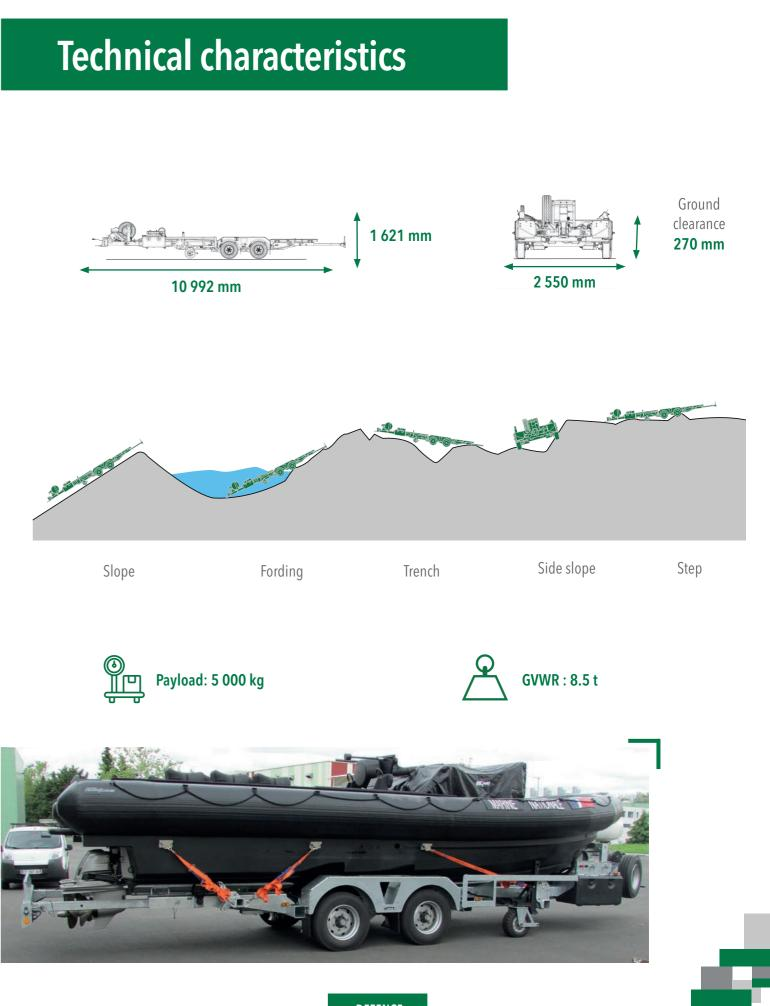
The airliftable trailer for fast boarding (**RPZ 5000**) is a **dirt track trailer** used to transport semi-rigid type boats by road, rail, sea or air.
