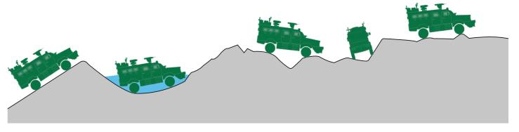
Step Slope Fording Trench Side Slope 30 % 60 % 600 mm 900 mm 400 mm
