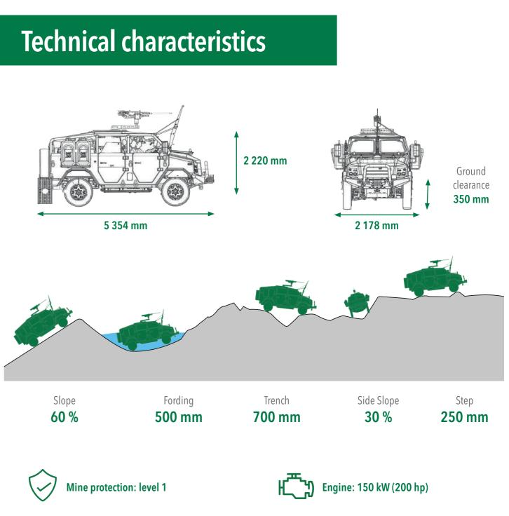
The **light-weight**, **fast**, **agile OUTFIELDER** is a 4x4 rapid intervention vehicle specifically designed for **special forces**, particularly for intelligence and infiltration operations.
