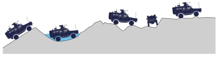
Side Slope Step Slope Fording Trench 60 % 30 % 600 mm 900 mm 400 mm
