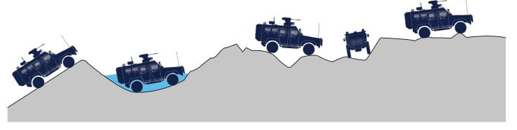
Side Slope Step Slope Fording Trench 60 % 30 % 600 mm 900 mm 400 mm
