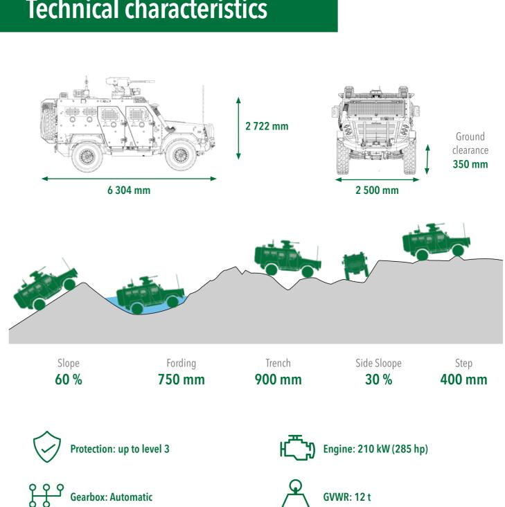
The **APCL** is a **protected rapid intervention** vehicle designed to operate in **extremely entangled areas and very varied terrains.** Its long range and all-terrain capability make it an extremely versatile vehicle.
