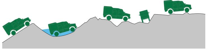
Side Slope Slope Fording Trench Step 40 % 30 % 800 mm 900 mm 400 mm
