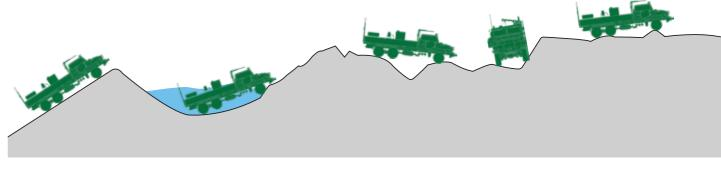
Step Slope Fording Side Slope Trench 60 % 800 mm 700 mm 30 % 350 mm
