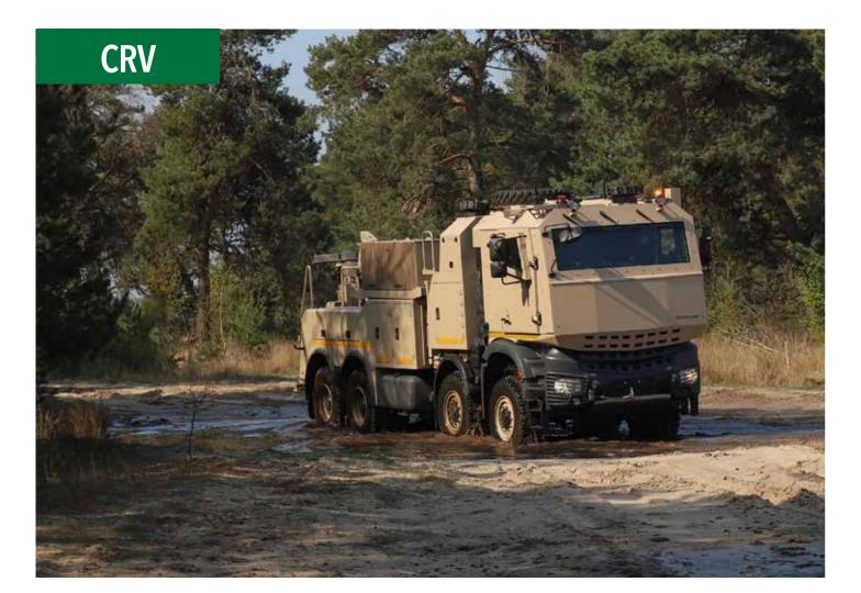
The **CRV** is a vehicle equipped with a **heavy towing system** used for the evacuation or extraction of brokendown wheeled vehicles.
