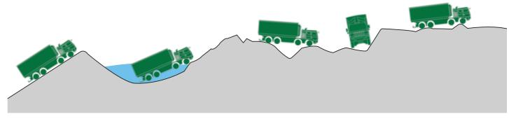
Side Slope Step Slope Fording Trench 30 % 40 % 800 mm 700 mm 350 mm
